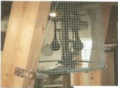
The governor in the centre automatically adjusts the gaps between the pairs of stones above according to the speed of the mill which varies with the speed of the wind. This ensures even quality of product once the initial gap has been set manually.
