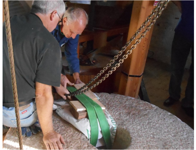
Getting the windmill ready for milling, lifting and cleaning the stones
